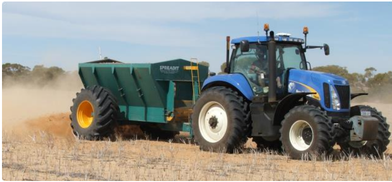
Figure: Clay spreading using a multi-spreader
