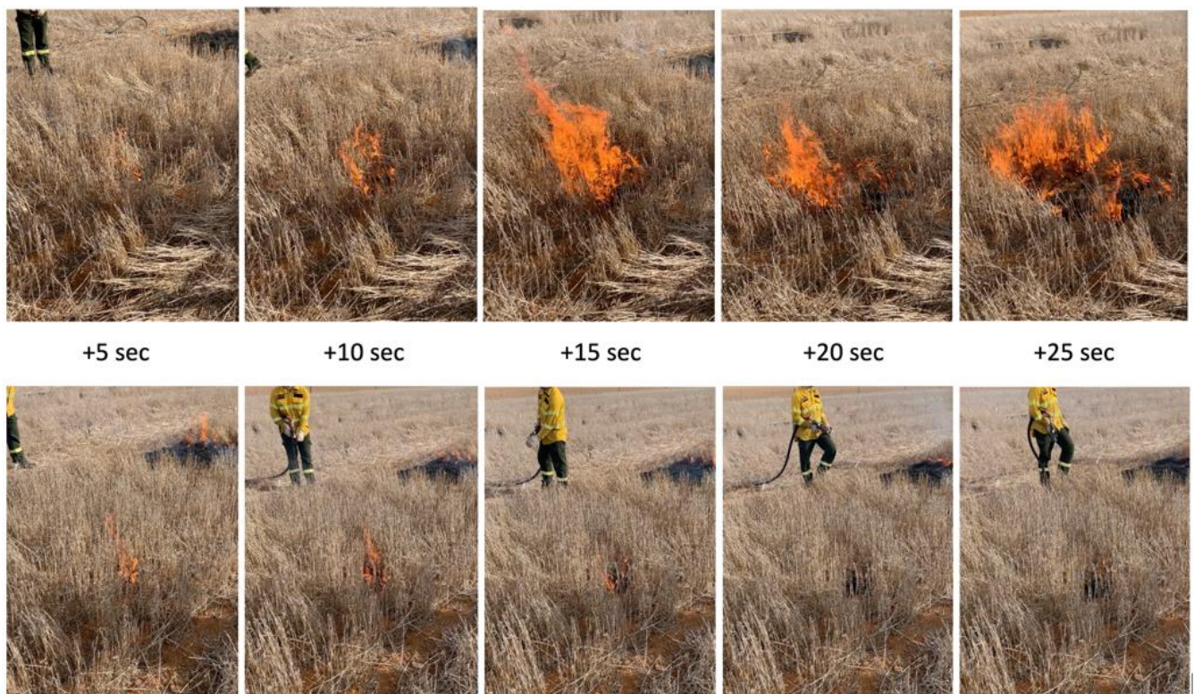
Figure 4a: The difference in the fire transmission rate between the best performing treatments and the Nil treatments was easy to see. (Nil above, Best below).
