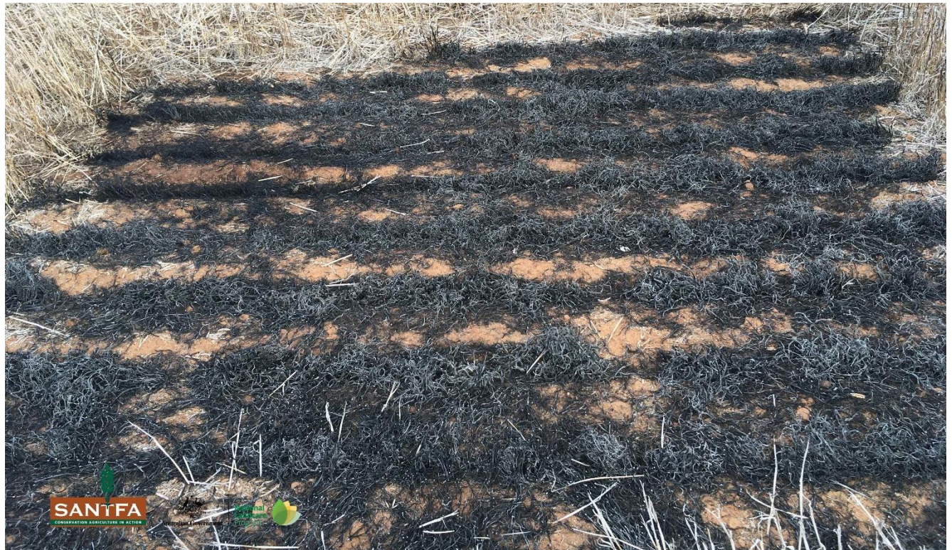
Figure 4b: Poor suppression. Plots that burned with the most intense fire resulted in the formation of char and ash. The presence of the white and grey ash is evidence complete combustion.
