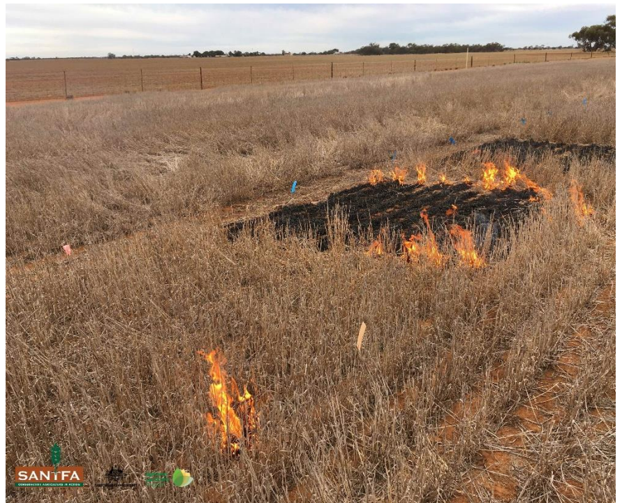
Figure 3: The ember attack was simulated by dropping a lit firelighter onto the up-wind side of every demonstration plot.
